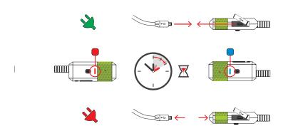
Before using your Twiins® HANDSFREE 2.0 device for the first time, you must charge the device completely. Connect the terminal (1c) to the provided USB charging cable (4) and then connect the cable to a USB charging port. While charging, the red LED light will switch on (1a) and it will change to blue once charging has been completed.
