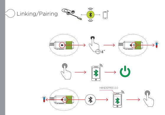
To use the Twiins® HANDSFREE 2.0, it's necessary to pair it to the Bluetooth® device you wish to connect it to (mobile phone, GPS navigator). While the device is switched off, hold the control button (1b) until the LED indicator (1a) begins flashing in Red and Blue. The mobile phone or GPS navigator will find the device under the name HANDSFREE 2.0. Select the HANDSFREE 2.0 device and, if necessary, enter the access code: 0000.
