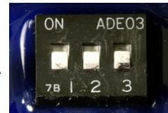
Map 2: switch n. 3 (see photo). This is the map for the engine equipped with Polini parts: Kit diameter 49 mm, gear up sets and variator.
