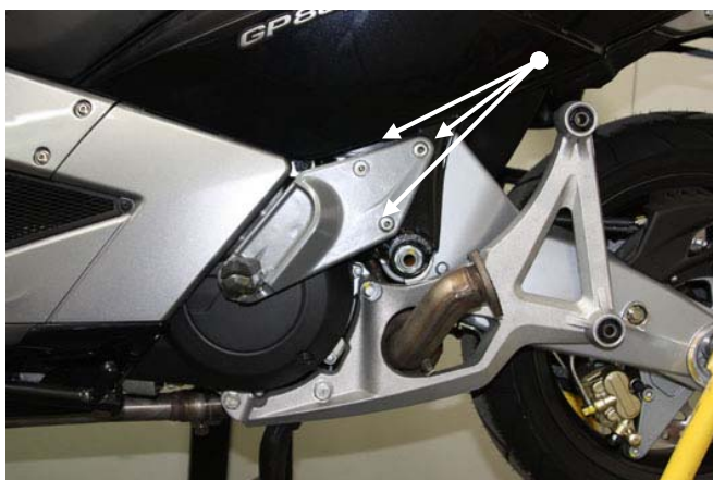
Smontare la pedana passeggero Remove passenger's footrest
