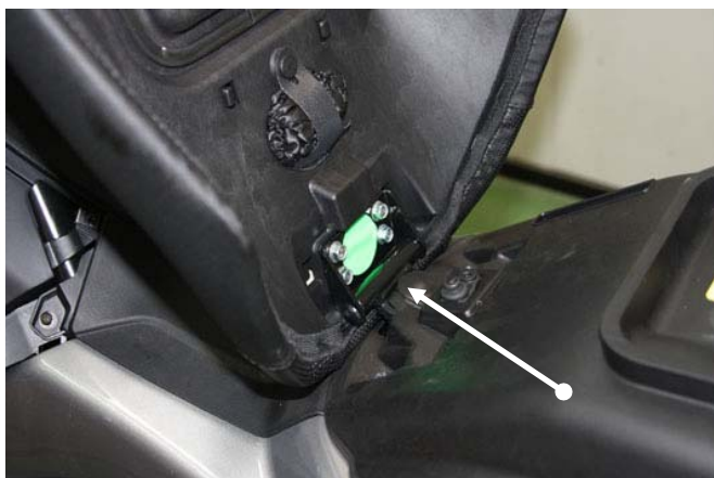
Smontare la sella attraverso gli appositi bulloni Remove the seat loosening the bolts shown in picture
