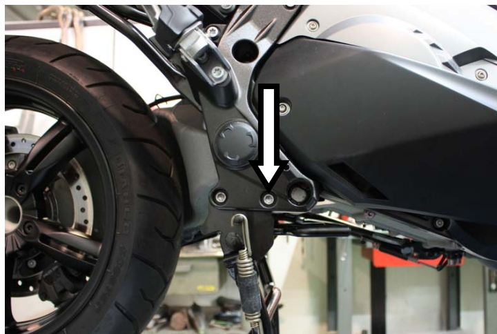
Sostituire la vite indicata con la TCEI M8x40mm fornita Replace the screw shown above with the M8x40mm socket head cap screw given in the fitting kit
